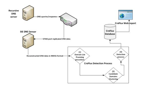
Figure 1. – Overview of CroFlux architecture
